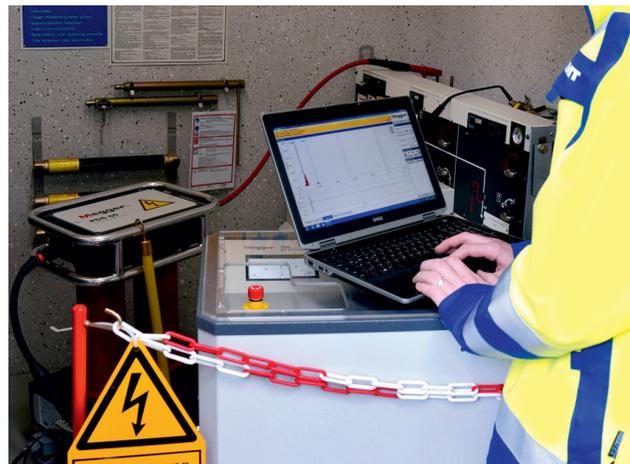
TDS 40 together with the PD detector PDS 60 in operation to test the quality of workmanship on a newly installed cable.
