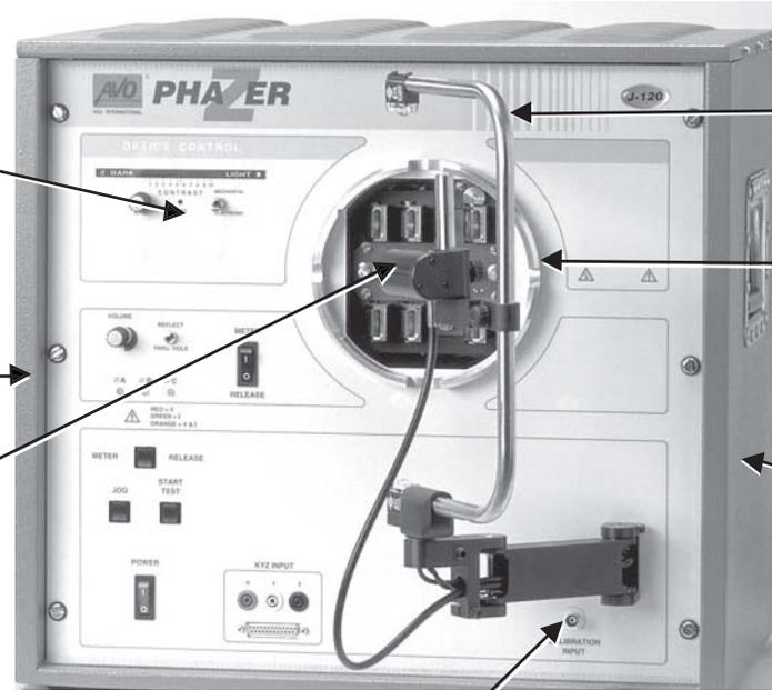
Easy-to-position C-Arm with through-hole sensor
