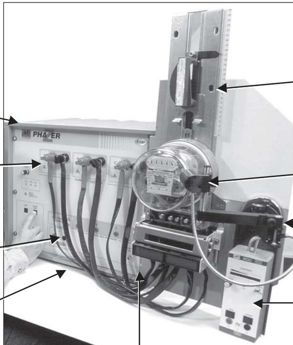
Improve efficiency of meter installation and removal using the optional IEC Meter Test Station.
