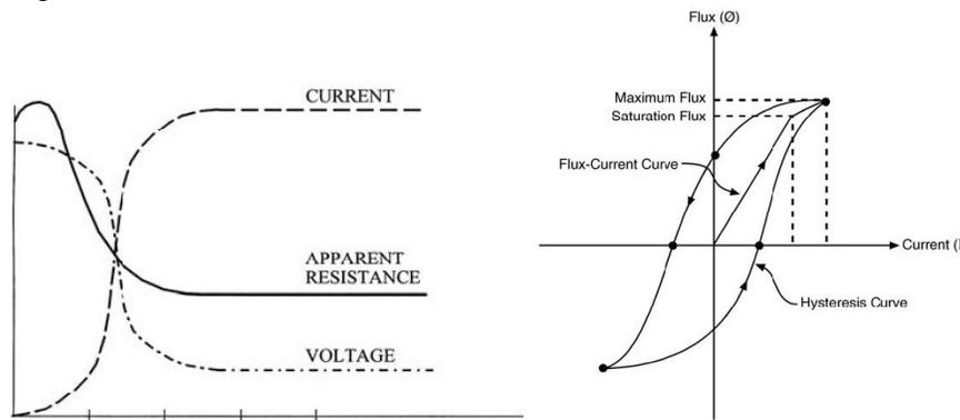
To the left: Illustration of Voltage, Current and Apparent resistance as function of time. To the right: A typical hysteresis curve for a magnetic material, e.g. transformer core. The Inductance L is proportional to the slope of the curve when current is changed
