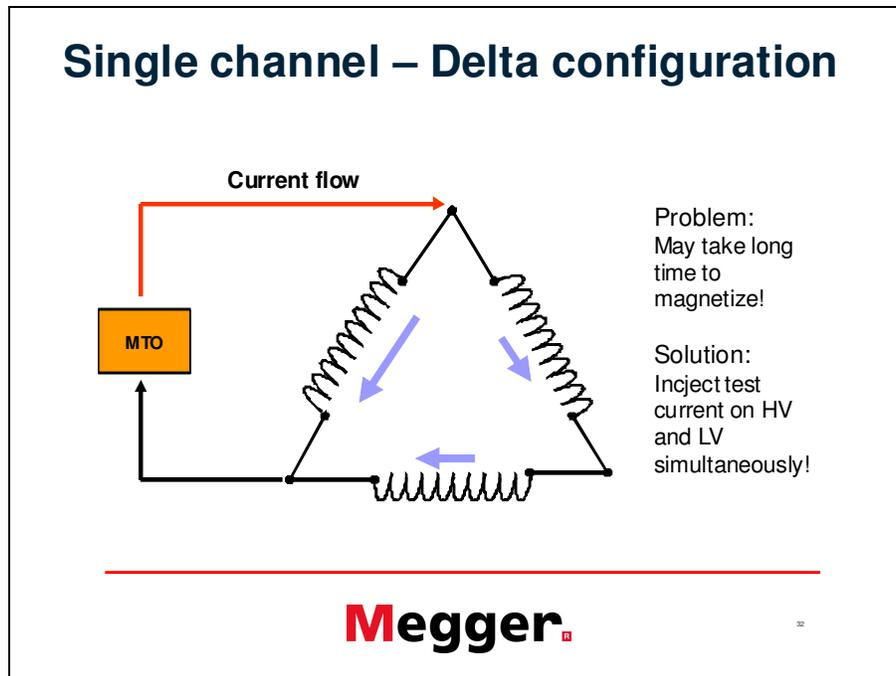
Figure 5. Closed delta winding
