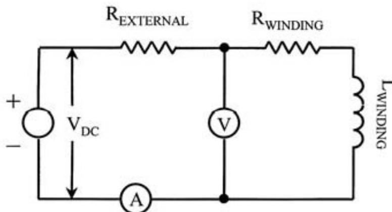
A DC test current is injected across the measured winding (-s), the voltage drop as well as the test current is measured and the resistance is calculated.
