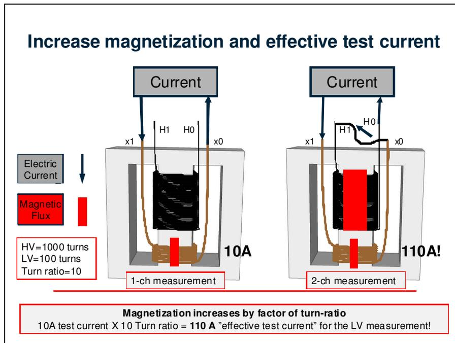
Figure 4. Amplification of magnetic flux by dual injection technique
