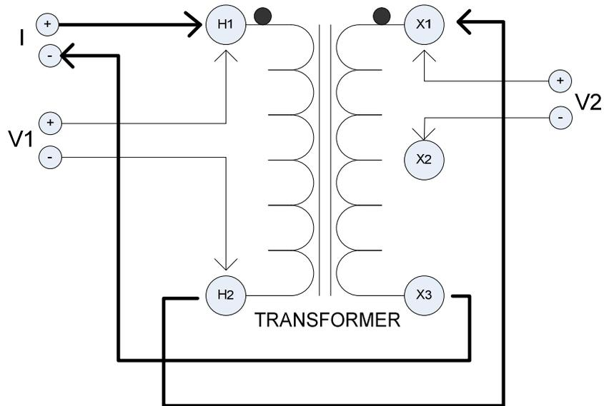
Figure 3. Measuring two windings simultaneously
