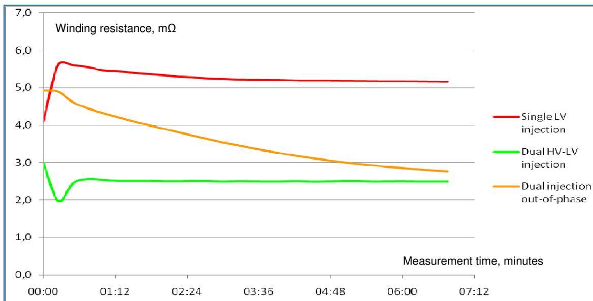
Figure 6. WRM on 200 MVA Ynd11 LV winding with different current injection techniques
