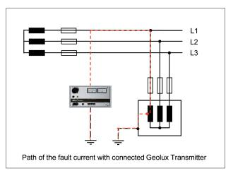
The integrated separation filter enables a direct galvanic coupling of up to 660 V AC and DC.
