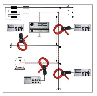
The operator follows the path of the signal current to the earth fault using inductive signal clamps (or an inductive contact sensor where cable bundling does not permit this). When the signal divides and can no longer be traced, he has found the earth fault.
